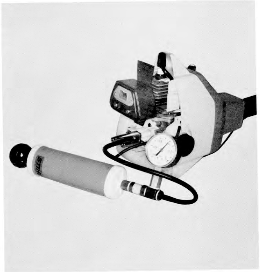
Diaphragm leakage test with vacuum pump
