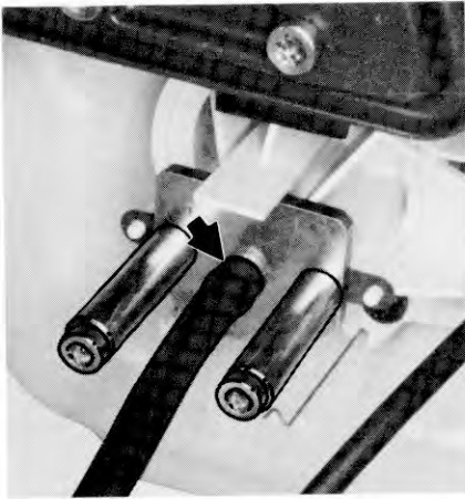
Tester's suction hose fitted on test flange nipple
