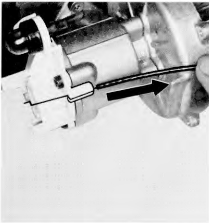
Withdrawing throttle cable
