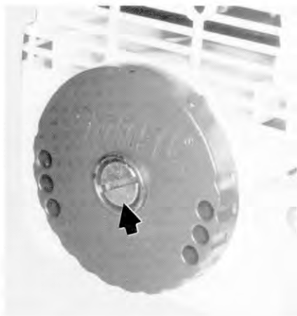
Filter cover mounting screw
