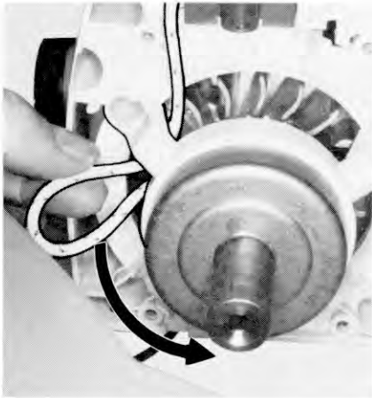
Winding rope onto rotor
