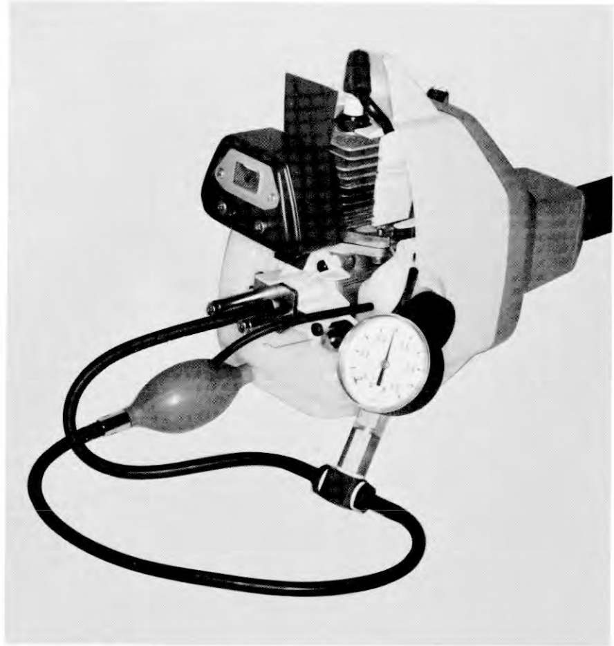
Pressure-testing the crankcase
