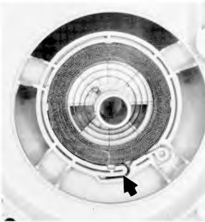
Rewind spring fitted in position
